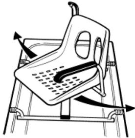
These seats rest across the rims of the bath and may be used in preference to a bath board as they provide a more supportive chair-type seat. They swivel to the left or right and many have a locking mechanism, which will secure the seat in a fixed position when the user is getting on and off. He/she sits to wash using a hand-held shower spray.
