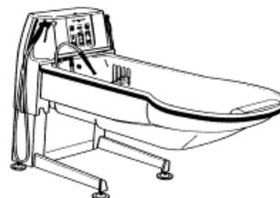
The height of these baths can be adjusted, either mechanically or electrically. They are designed to reduce the need for a carer to bend over the bath if the person needs assistance. The bather may be able to step into the bath at its lowest level and then be raised to a convenient height. However, remember that the water usually needs to drain away before the bather can get out. These baths are not often used in a domestic setting.
