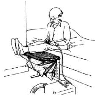
These are powered devices that attach to the bed frame and require the user to sit on the edge of the bed with his/her feet on the floor in front of the device. They work on the principle of a platform that raises through an arc of 90°, lifting the legs of the user to a position just beyond the horizontal, level with the mattress. From this position the user can slide his/her legs off the platform and onto the bed.
