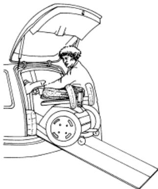
Different types of ramps can be used to get a wheelchair or powered vehicle into the back of the car. Once again the user will generally need help to do this. If a wheelchair is to be taken up a ramp into the back of the car, the hatch should be level-access, i.e. without a boot sill. If there is a sill, an alternative method will have to
