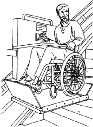
These powered lifts are mounted on stair-fixed tracks that follow the line of the stairs. The track may be on one or both sides of the stairs. This particular type has a platform large enough to carry a wheelchair and its user. Some platforms fold down from against the wall where they are stored when not in use, others rest in a floor recess when not in use. Wide stairs are needed because of the size of the platform.
