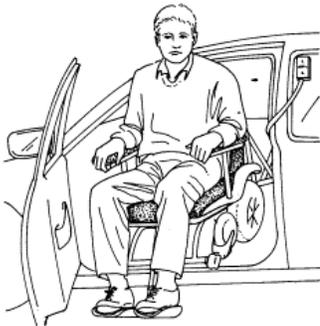
This system uses a seat which acts as both a wheelchair seat and a car seat, The seat swivels out of the car and slots onto a wheelchair base which is stored in the boot of the car while the passenger is transported in the car. It eliminates a transfer from one seat to another between wheelchair and car..
